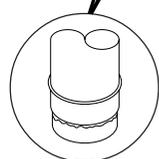
Use a listed Category III vent adapter to connect the flue collar to the vent system. Use Category III vent pipe for the entire length of the exhaust pipe.
