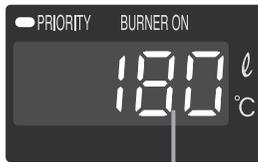
Flow meter setting will be flashing (ex. 180L (48gallons))
