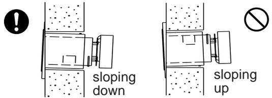
3) Install with the proper length protruding through the wall
