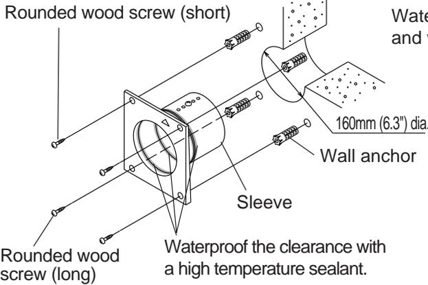
Waterproof the clearance between the sleeve and wall hole with a high temperature sealant.
