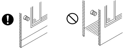
2) Install the vent terminal with a downward slope
