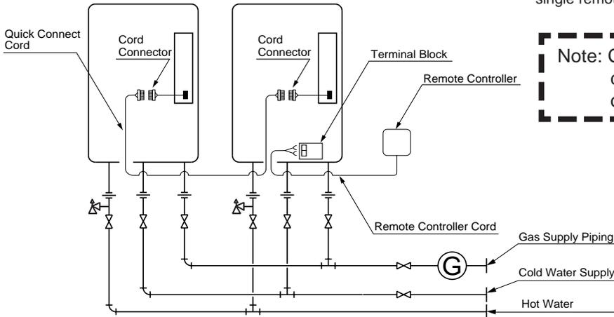
Note: Connect the remote controller to only one of the devices.
