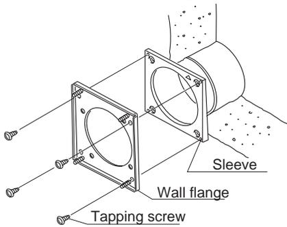
\* The proper flange orientation depends on the desired orientation of the vent terminal.
