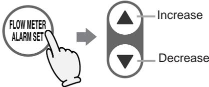
Choose the flow meter alarm setting from the following options: 38 - 260 L (10 - 60 gallons) (In 20 L (5 gallons), 300 L (80 gallons), 340 L (90 gallons), 380 L (100 gallons), 990 L (262 gallons).)
