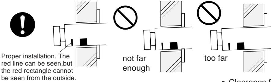
Proper installation. The red line can be seen, but the red rectangle cannot be seen from the outside.
