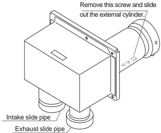
At this point, make sure the supply and exhaust slide pipes have been inserted into vent terminal.
