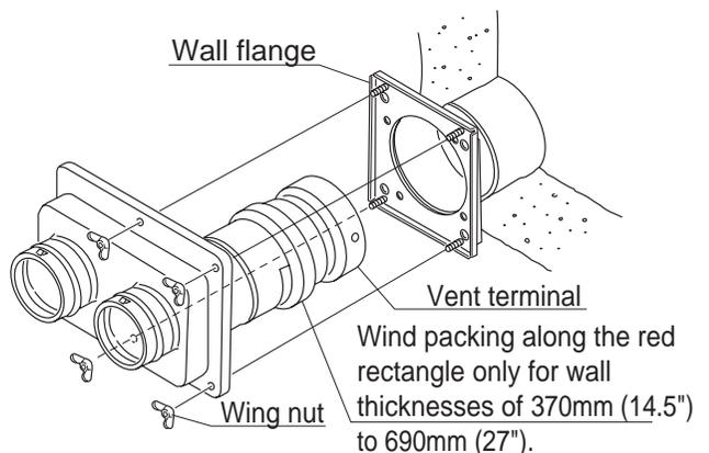
\* Installation pattern (3) yields a clearance between the vent terminal and the wall surface. Fill this clearance with a high temperature sealant.
