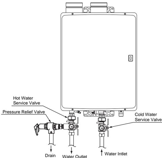
\* Isolator valve kits may be purchased as an accessory from Noritz (Part #IK-WV-2). They allow for one man full diagnostic testing and easy flushing of the system.
