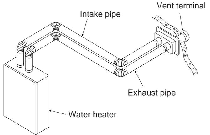
Connect the vent pipe to the vent terminal as follows:
