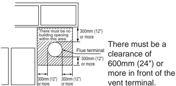
• This restriction will not be applied to an area where an effective shield makes a clearance of 600mm (24") or more in front of the exhaust outlet.
